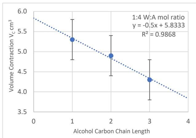
**Graph 2.** A carbon chain length vs  $V_c$  (1:4) W : A mol ratio
