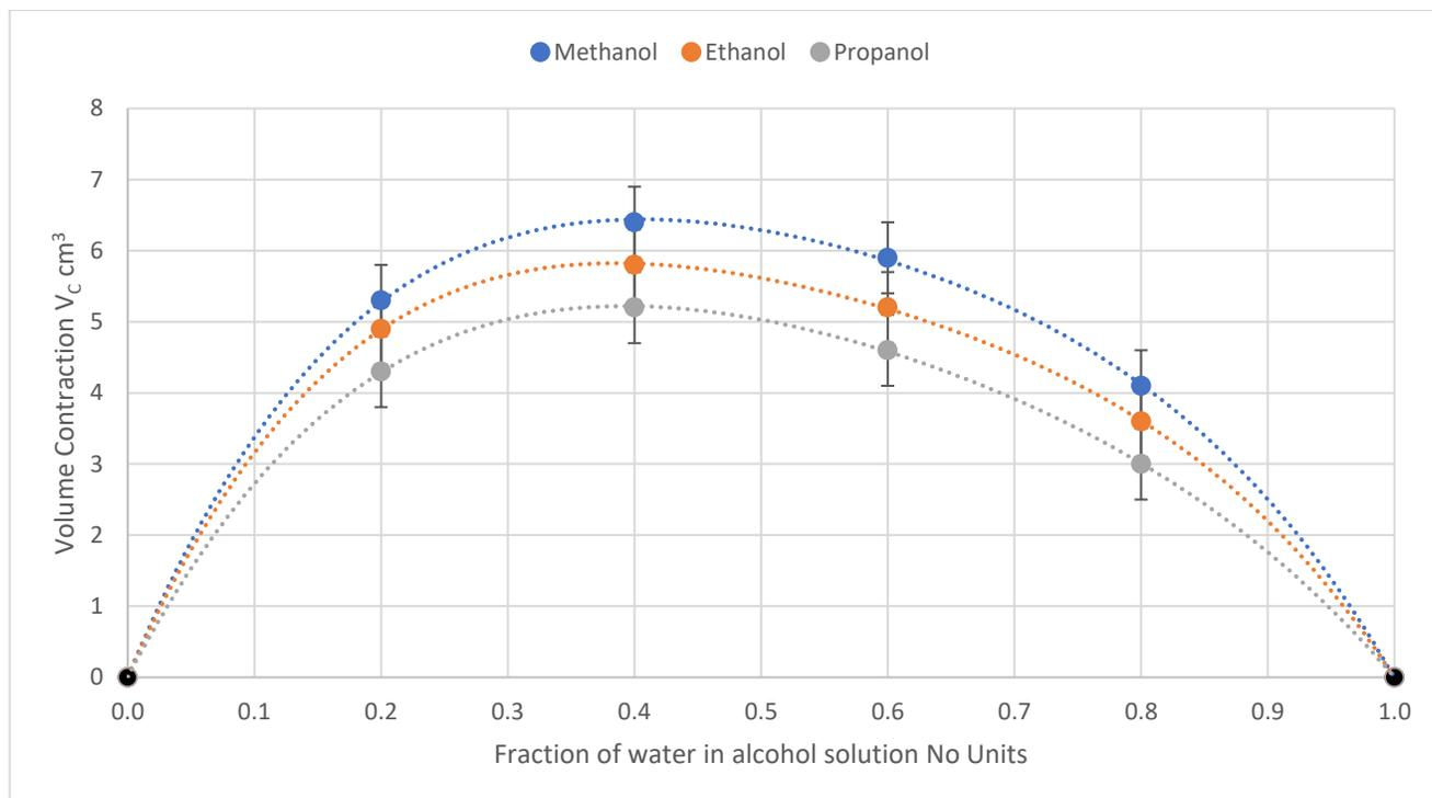
**Graph 1.** Volume Contraction of Methanol, Ethanol, and Propanol depending on W : A ratio
