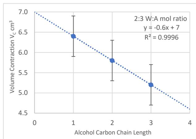
**Graph 3.** A carbon chain length vs  $V_c$  (2:3) W : A mol ratio
