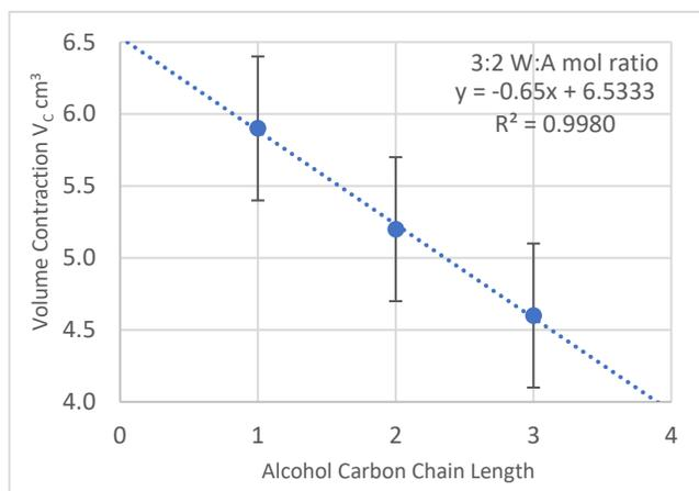
**Graph 4.** A carbon chain length vs  $V_c$  (3:2) W : A mol ratio
