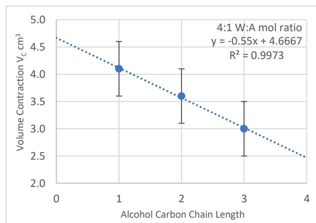
**Graph 5.** A carbon chain length vs  $V_c$  (4:1) W : A mol ratio
